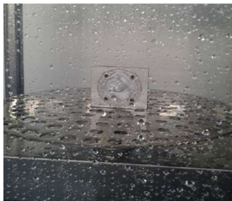
Testing under water jet
